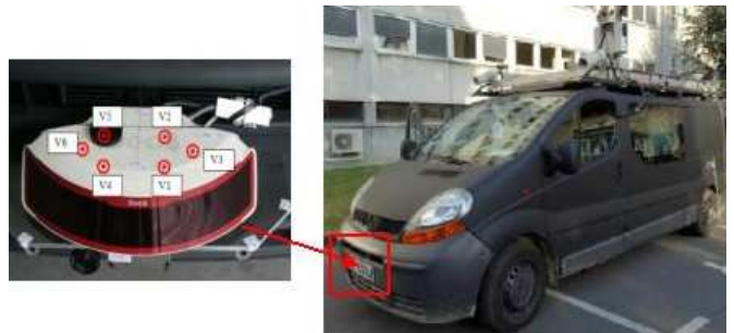
Figure 2: Left, the IBEO ALASCA XT Laserscanner and the Marlin 146-C camera. Right, the IGN test vehicle.
